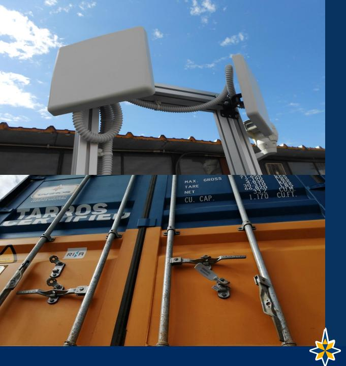
Antennas allow detection of RFID seals placed on the container to control access
