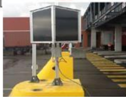
Automatic Gate-in at the terminal thanks to RFID antennas
