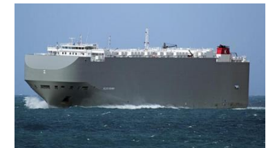
Helios Highway (2015) 7,500 ceu Post-Panamax Length 200m / Beam 35.4m Draft 10.6m
