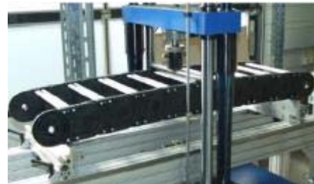
Bending moment tests
