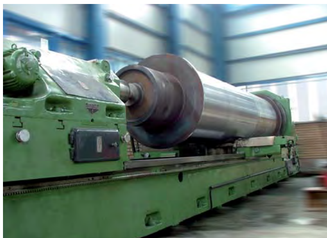
Heavy Lathe Machine Machining line For manufacturing of heavy duty cranes drums
