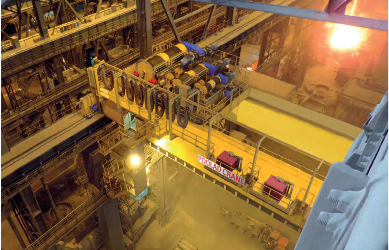
Scrap Charging Crane 110/40/10 Ton x 30 meters
