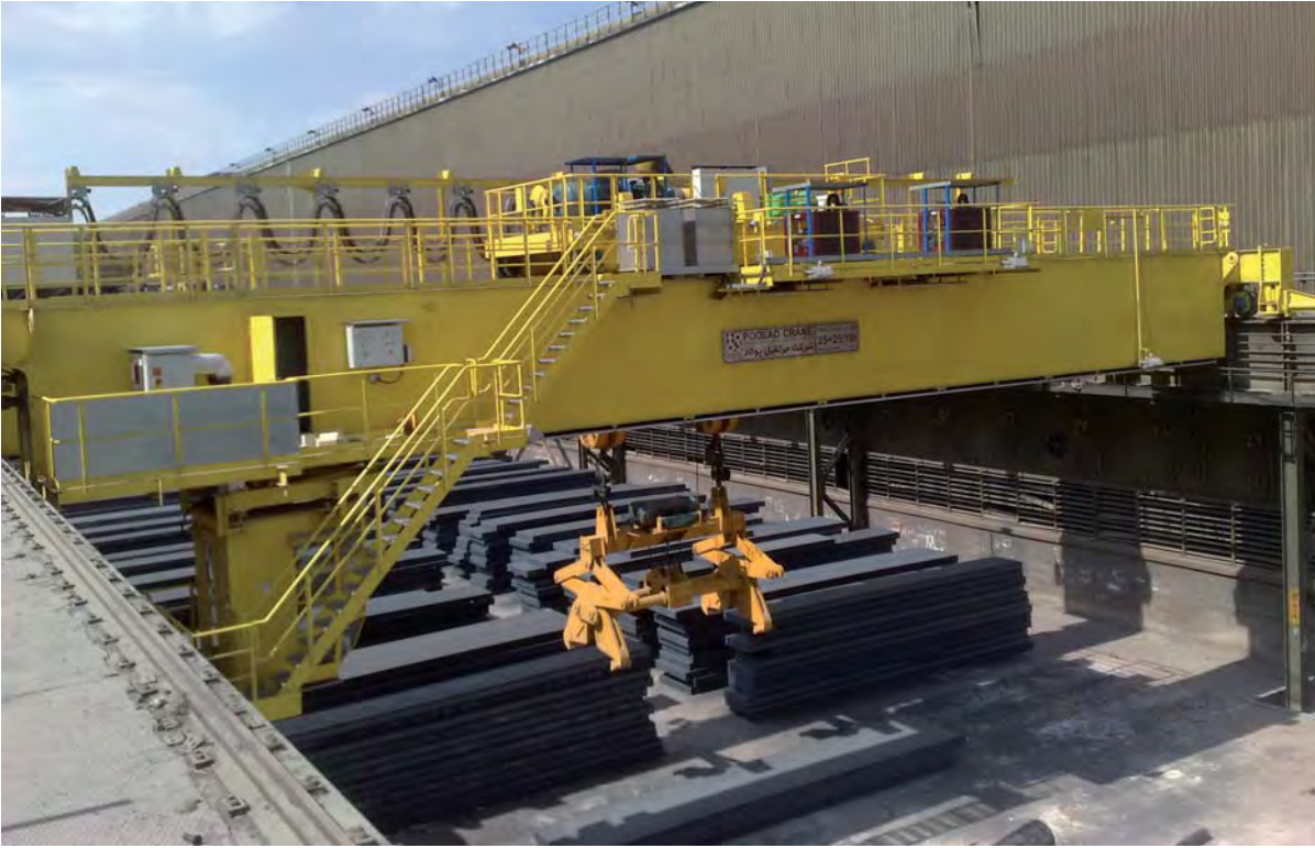
25+25(50)/10 Ton x 28m - Slab Tong Crane
