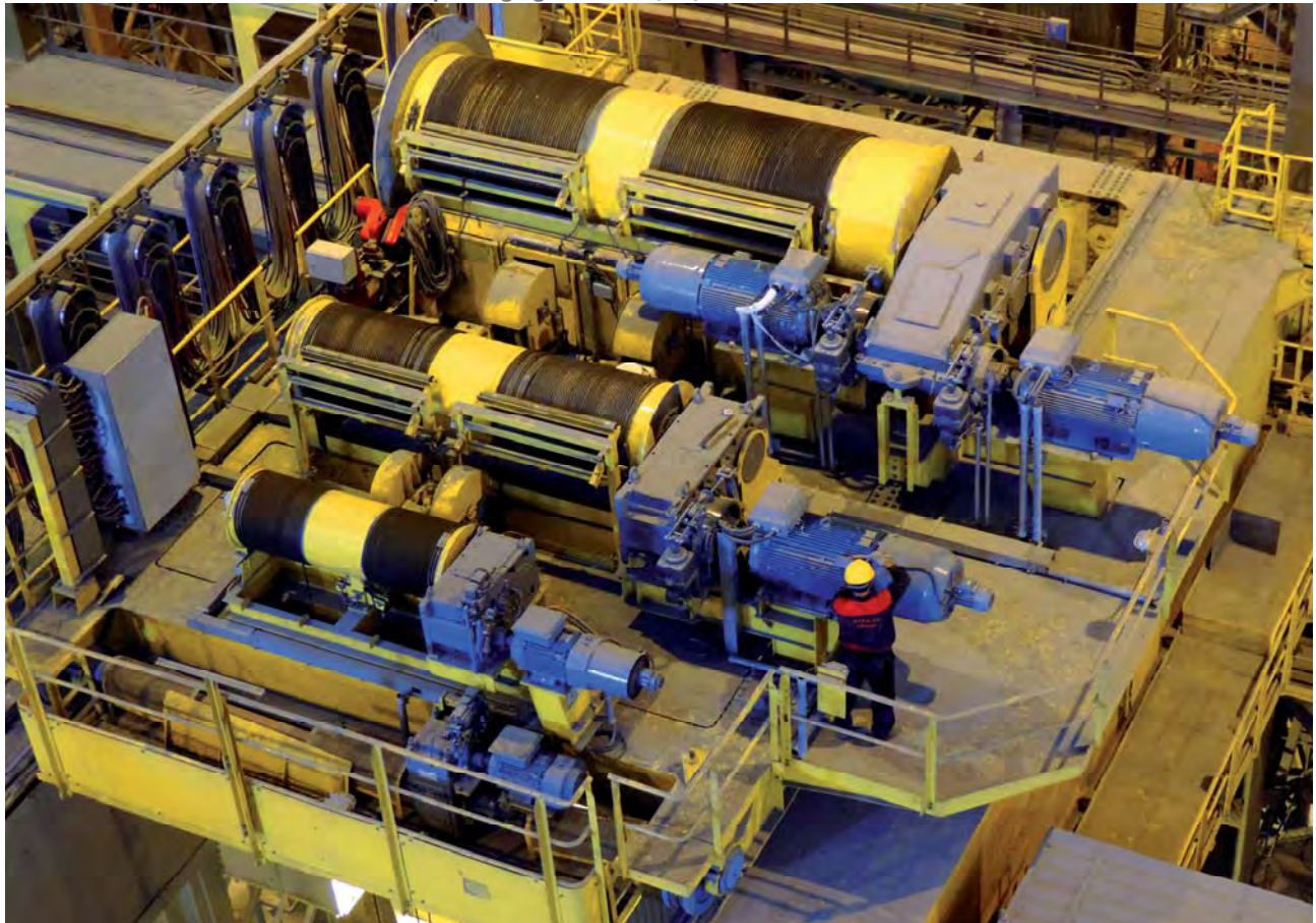
Scrap Charging Crane 110/40/10 Ton x 30 meters
