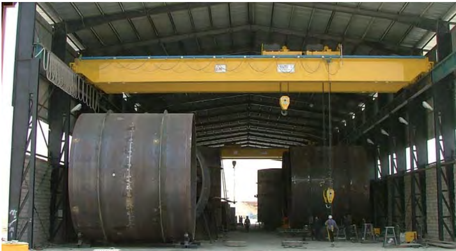
Gotvand Dam Kian Payab EOT Cranes 2x20(40)Ton 2 Sets
