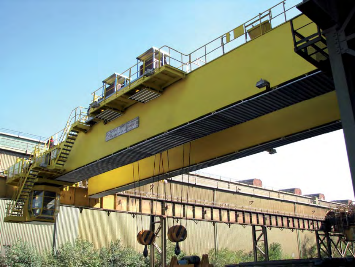
25+25(50)/10 Ton x 28m - Slab Tong Crane
