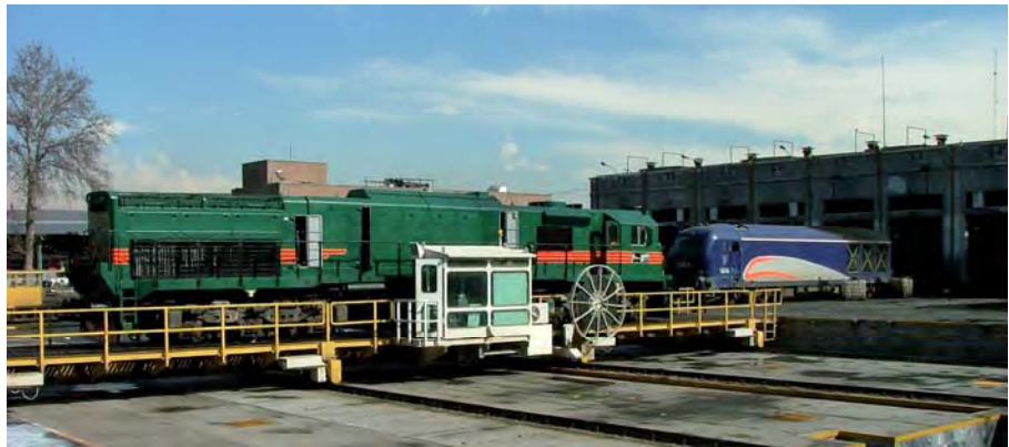
IRI - Railway Company Locomotive Transfer Table 250-Ton
