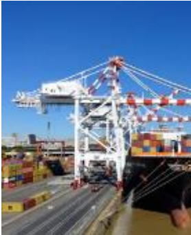
Buenos Aires, Argentina Boom extension and relocation of two non-Kalmar STS cranes ▪ 6-metre boom extension
