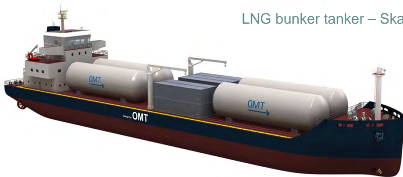
LNG bunker tanker – concept design, Helsingborg
