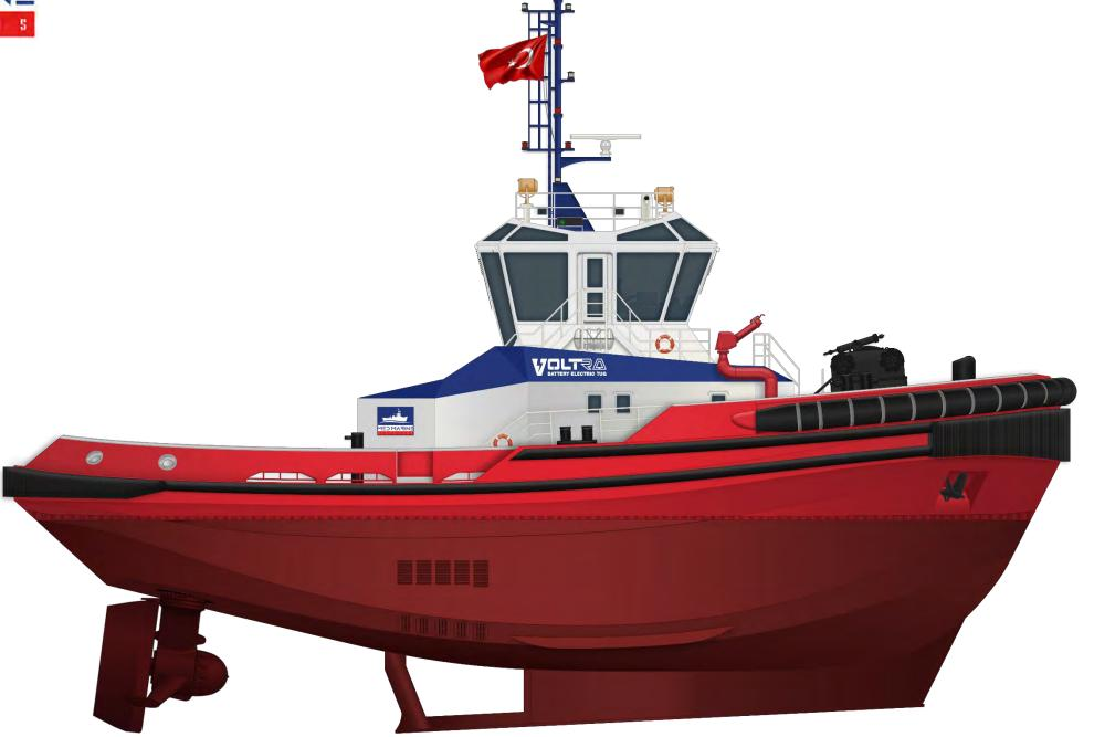
VoltRA 3000 Battery Electric Tug series are designed by Robert Allan, driven by 2 x 2525 kW propulsive power and 5000 kWh battery pack capacity max. The vessel is equipped with a forward towing winch, an aft towing winch, an aft towing hook and internal and external firefighting system. Two (2) gensets will be installed in case of emergency and firefighting.
