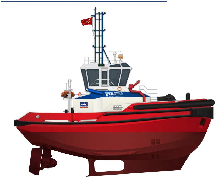
VoltRA 2300 Battery Electric Tug series are designed by Robert Allan, driven by 2 x 1850 kW propulsive power and 3390 kWh battery pack capacity max. The vessel is equipped with a forward towing winch, an aft towing hook and internal and external firefighting system. Two (2) gensets will be installed in case of emergency and firefighting.
