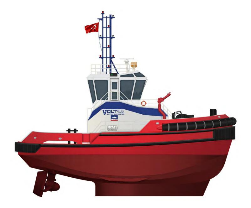
VoltRA 2100 Battery Electric Tug series are designed by Robert Allan, driven by 2 x 1400 kW propulsive power and 2900 kWh battery pack capacity max. The vessel is equipped with a forward towing winch, an aft towing hook and internal and external firefighting system. Two (2) gensets will be installed in case of emergency and firefighting.
