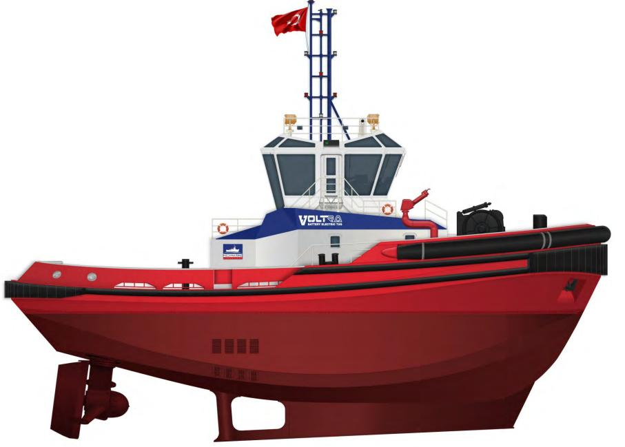
VoltRA 2800 Battery Electric Tug series are designed by Robert Allan, driven by 2 x 2525 kW propulsive power and 4500 kWh battery pack capacity max. The vessel is equipped with a forward towing winch, an aft towing winch, an aft towing hook and internal and external firefighting system. Two (2) gensets will be installed in case of emergency and firefighting.
