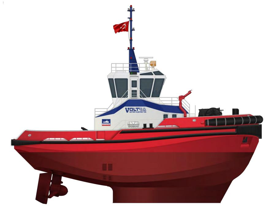
VoltRA 2500 Battery Electric Tug series are designed by Robert Allan, driven by 2 x 2350 kW propulsive power and 4295 kWh battery pack capacity max. The vessel is equipped with a forward towing winch, an aft towing winch, an aft towing hook and internal and external firefighting system. Two (2) gensets will be installed in case of emergency and firefighting.
