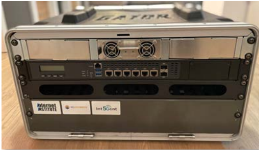
Integrated Private 5G System COTS Server, 48V Modular Power Supply
