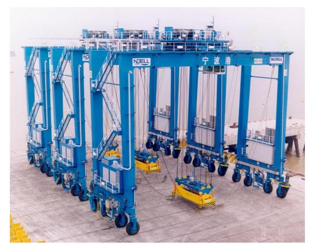
Hoist: *Motor type:* DRKF 315 L-6bbbT *Power:* 1 x 210 kW
