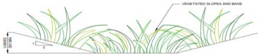
BIO RETENTION SWALE CROSS SECTION - TYPE A SCALE 1:20
