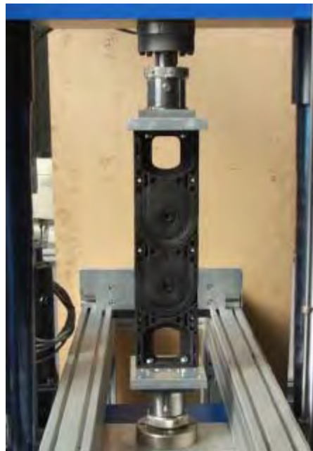
Push-pull forces tests
