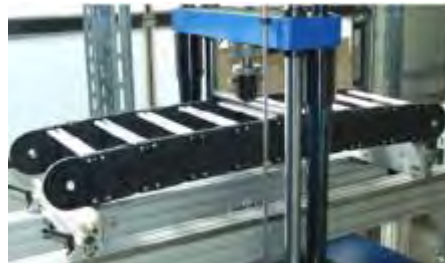
Bending moment tests
