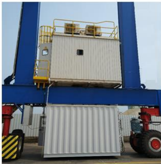
Battery housing mounted under sill beam
