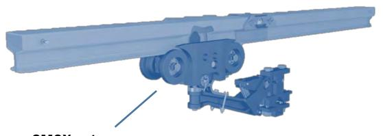
**SMGX antenna** installed at the current collector trolley
