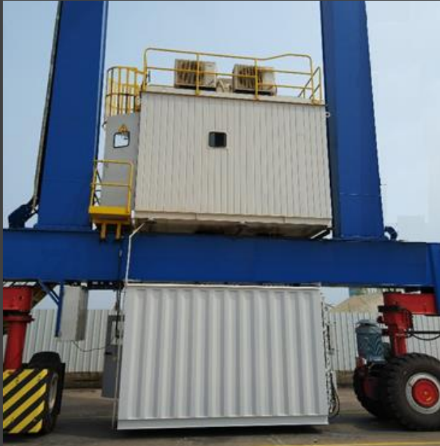
Battery housing mounted under sill beam
