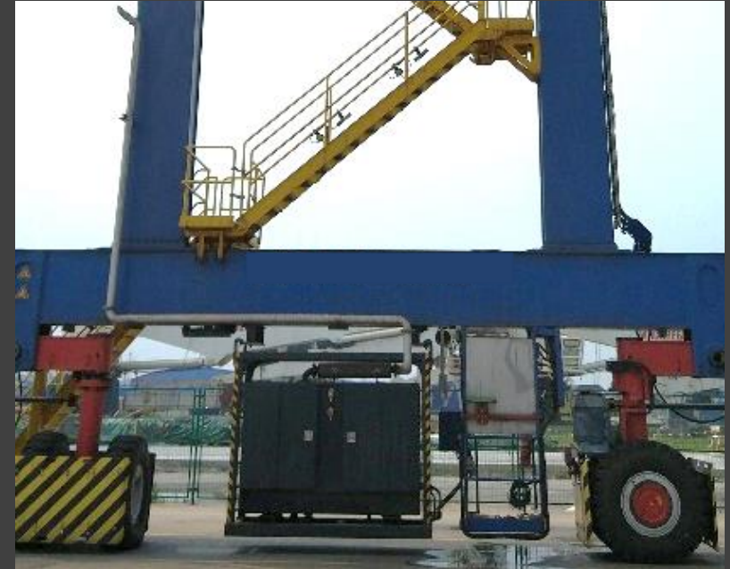
Small diesel genset mounted under sill beam
