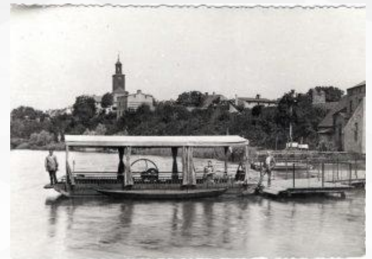
Electrical, catenary-powered Ferry on Straussee near Berlin, Germany in 1915
