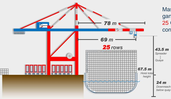
Massive Super-Post-Panamaxgantry cranes capable of handling 25 Container rows and 11 standard container tiers on deck
