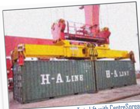
Separating Twin Lift with CentreSpread
