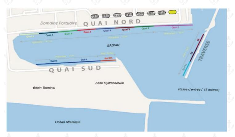
**North wharf:** (1.250m quaywall): 8 berths > breakbulk, bulk, roro & containers
