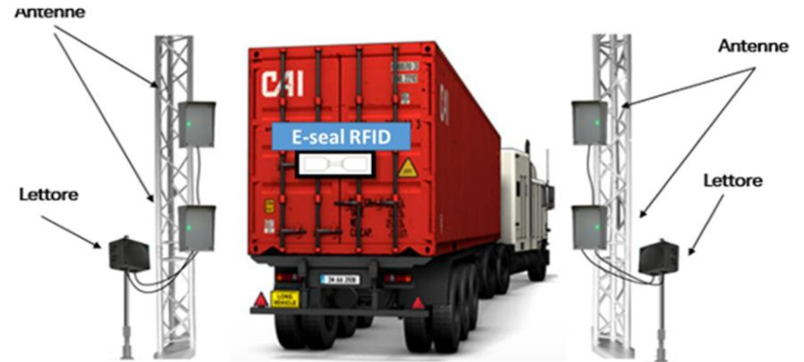
Example of automated port entry using RFID technology. The system consists of two readers and two antennas per reader. When the container crosses the gate, the reader reads the tag / e-seal rfid
