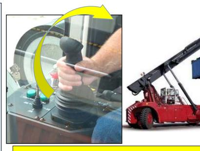
Through this (selectable) function the driver does not manage anymore the throttle when lifting-lowering the load.
