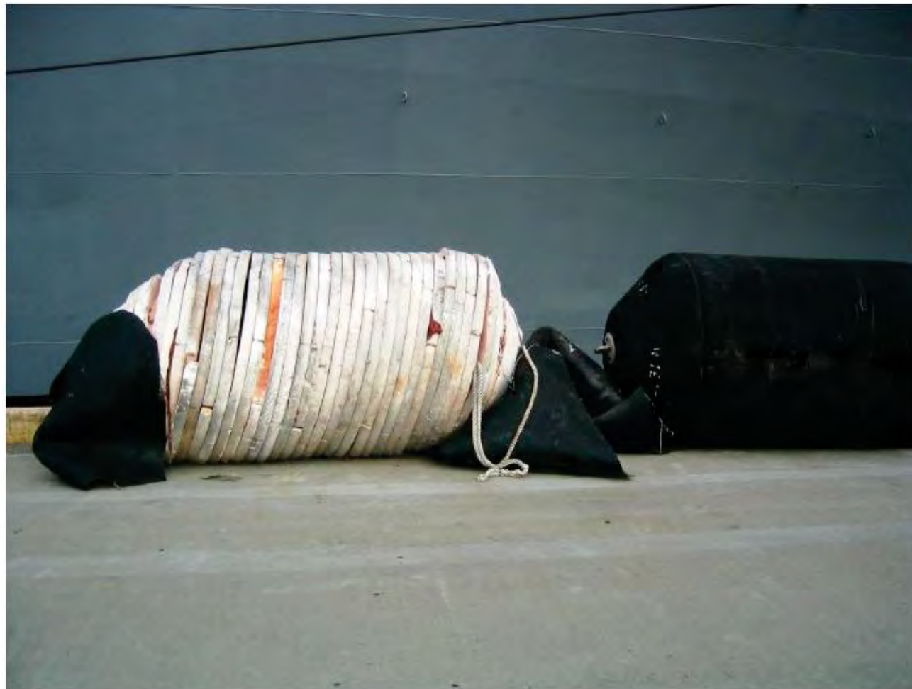
Inferior Non laminated foam disc construction
