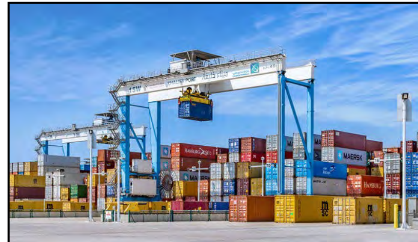
Automated Stacking Cranes (ASC & ARMG)
