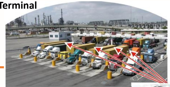
Automatic Gate-in at the terminal thanks to RFID antennas
