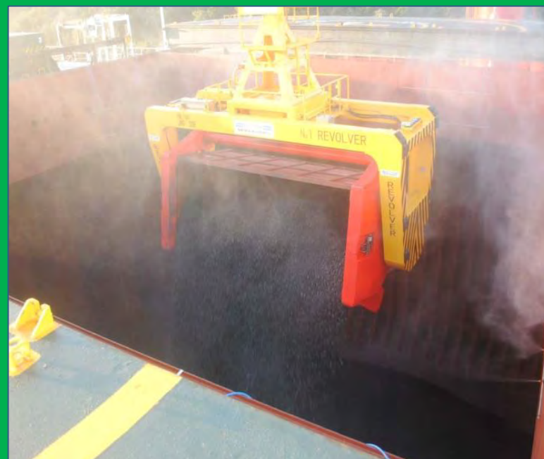
MISTING SYSTEM ON
