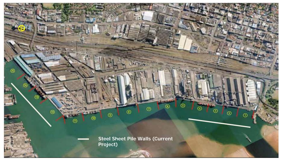
Replace old steel sheet pile berths 1-4, and 12-14, with new deep water berths : Provide infrastructure to sustain existing port operations and cater for growth in cargo volumes
