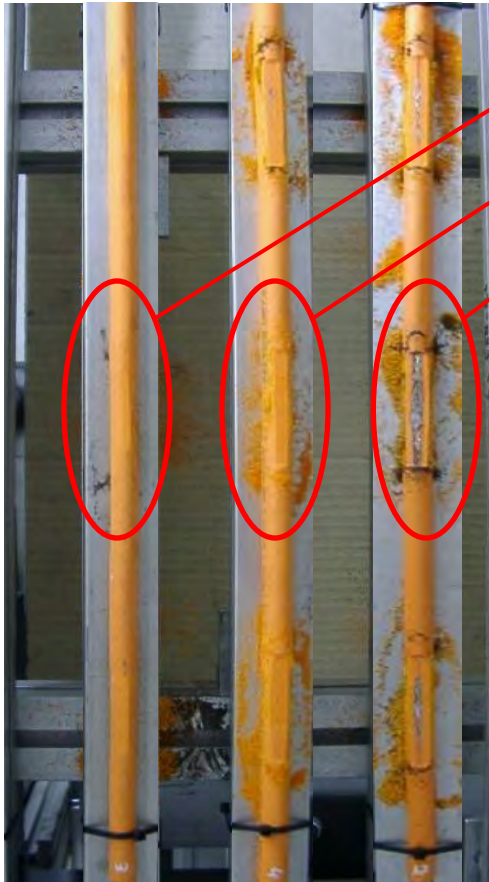
Jacket wear test at our Kabelschlepp Test Area
