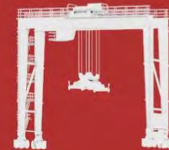
Rubber Tyre Gantry (RTG)
