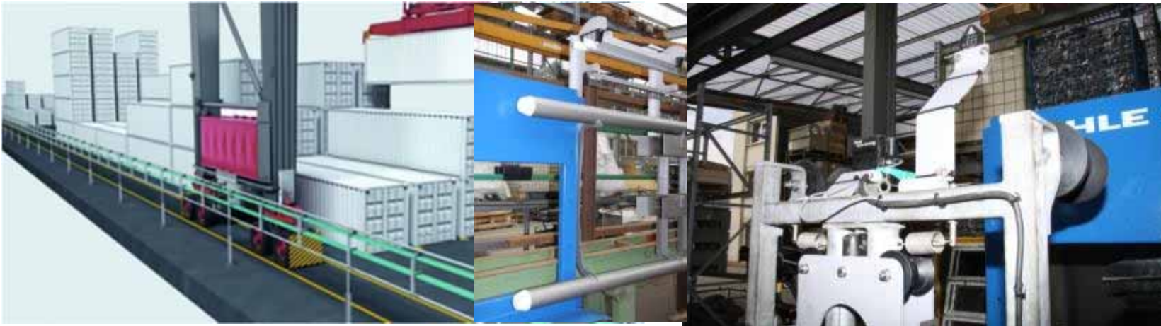
The Busbar power connection converts the RTGs to fully electric operation. Image: Konecranes
