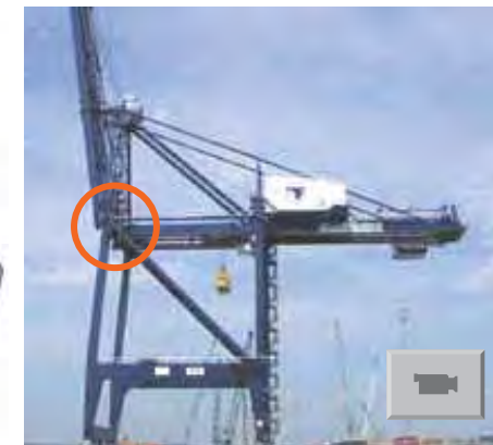
Hinge clutch at hinge point incl. limit switch
