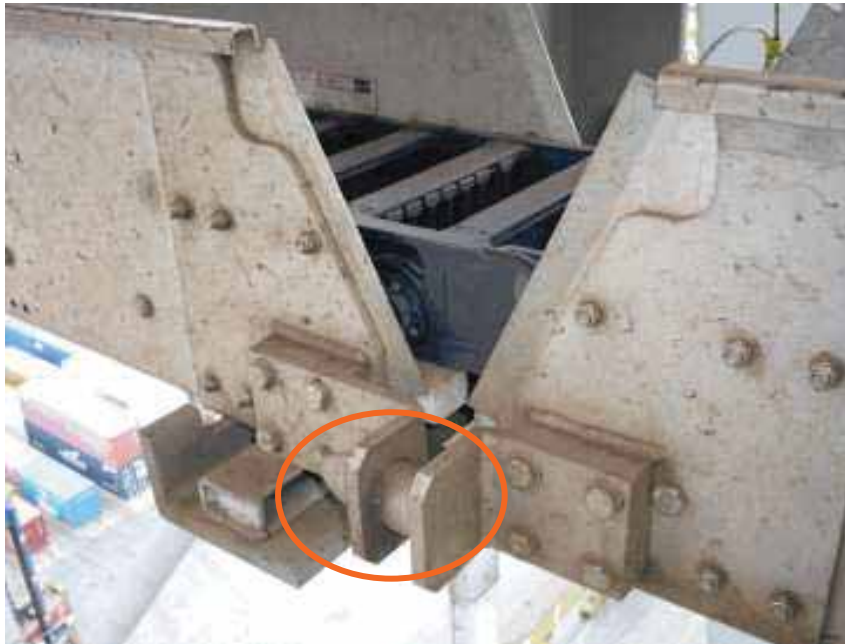
Hinge clutch at the hinge point with bolts and holes to get a safe adjustment after bringing down the boom
