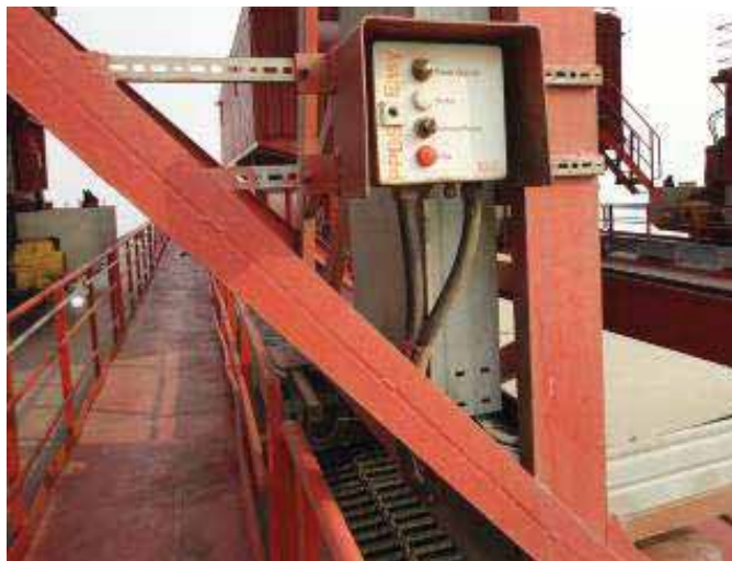
Push-/Pull-force monitoring with the igus® PPDS System
