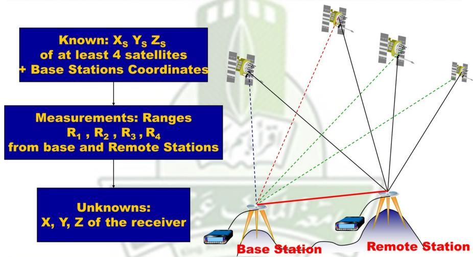
Positioning Accuracy: few meters (one sigma)
