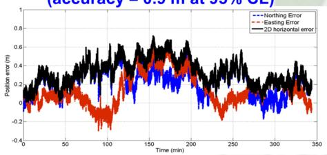
PPP-based GNSS solution errors (accuracy = 0.2 m at 95% CL)
