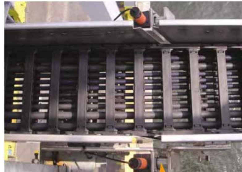
Hinge clutch at hinge point including limit switch
