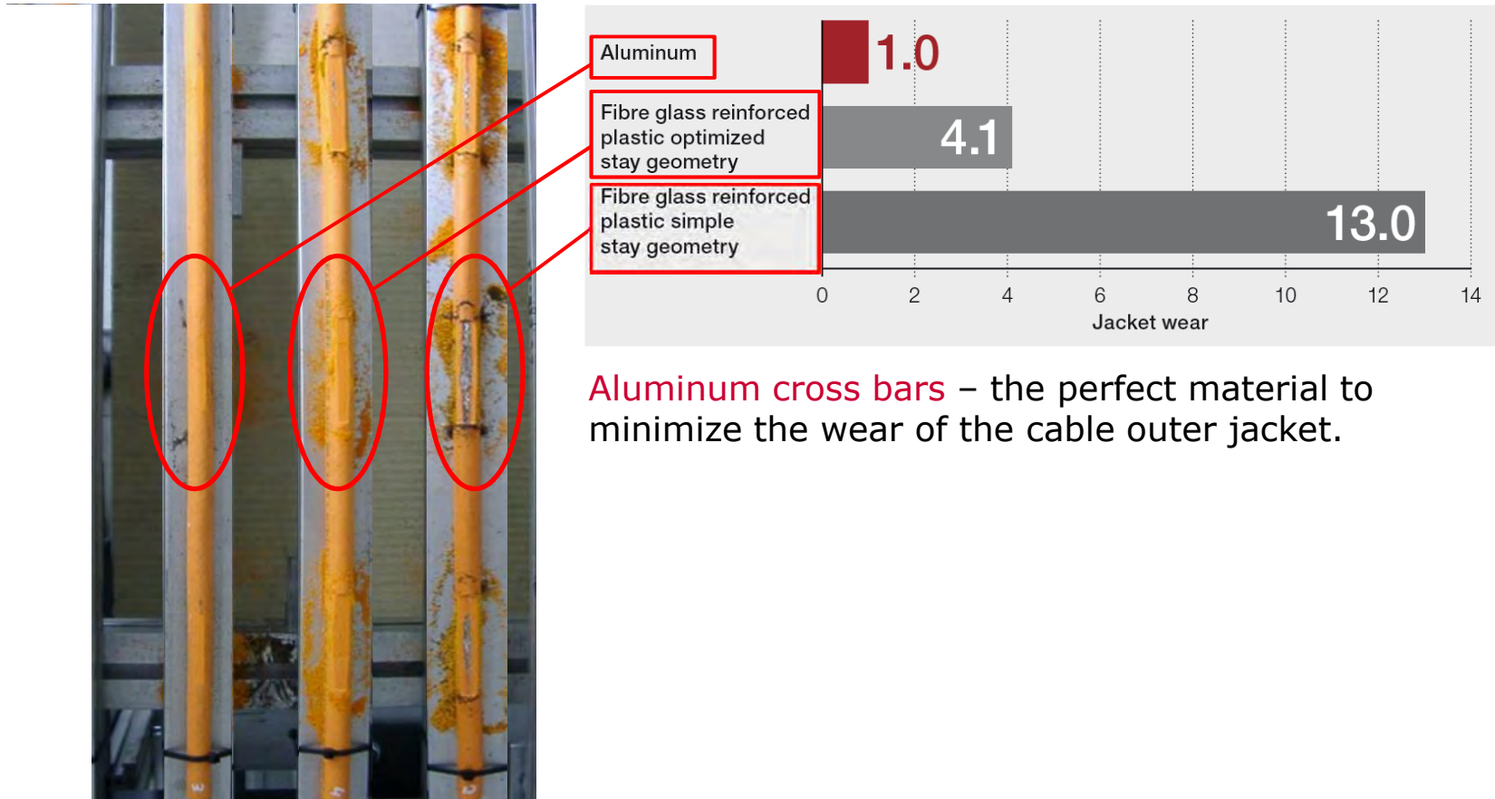
Jacket wear test at our Kabelschlepp Test Area
