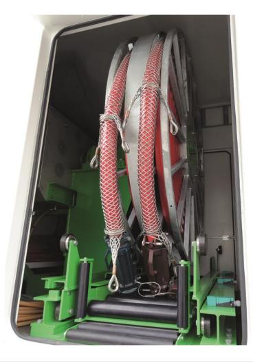
The feed of the onshore power supply for container vessels is realised for example by the installation of a 40 ft. HC-container in the bottom storage row.
