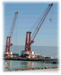
**1 Gottwald HMK7608 Crane** Max lifting capacity: 140 Tons
