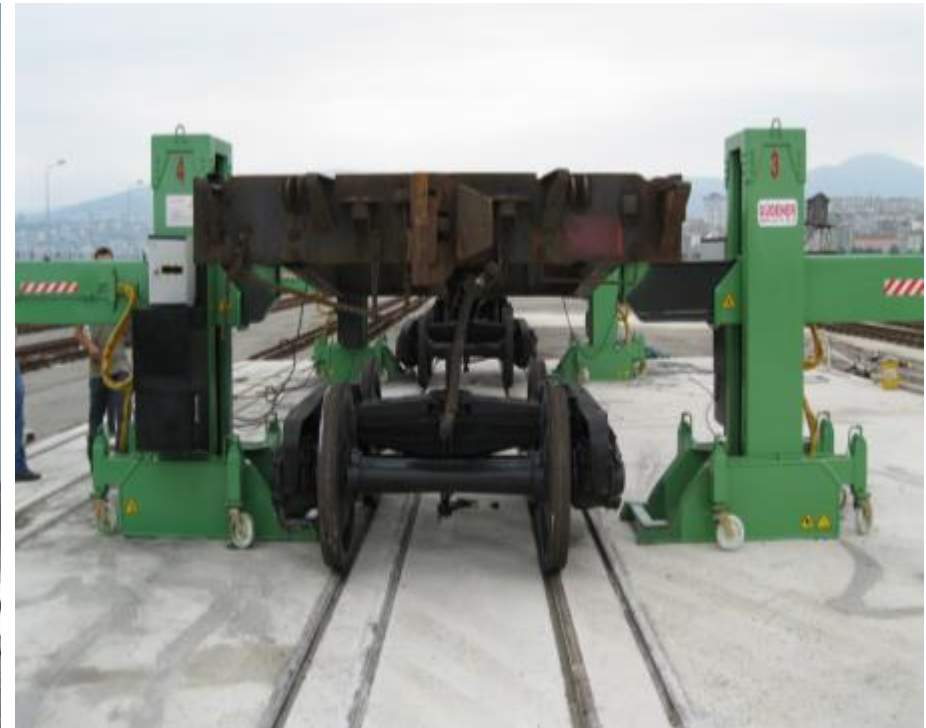
Bogie Changing Gantry
