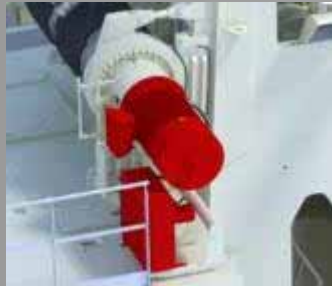
Easily accessible hoist driven through AC motors with optional enclosure
