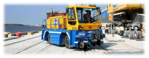
Rail wear and track maintenance costs are also reduced, due to the lighter vehicle weight, traction by the rubber wheels and the specially designed rail guide wheels of the LOCOTRACTOR.
