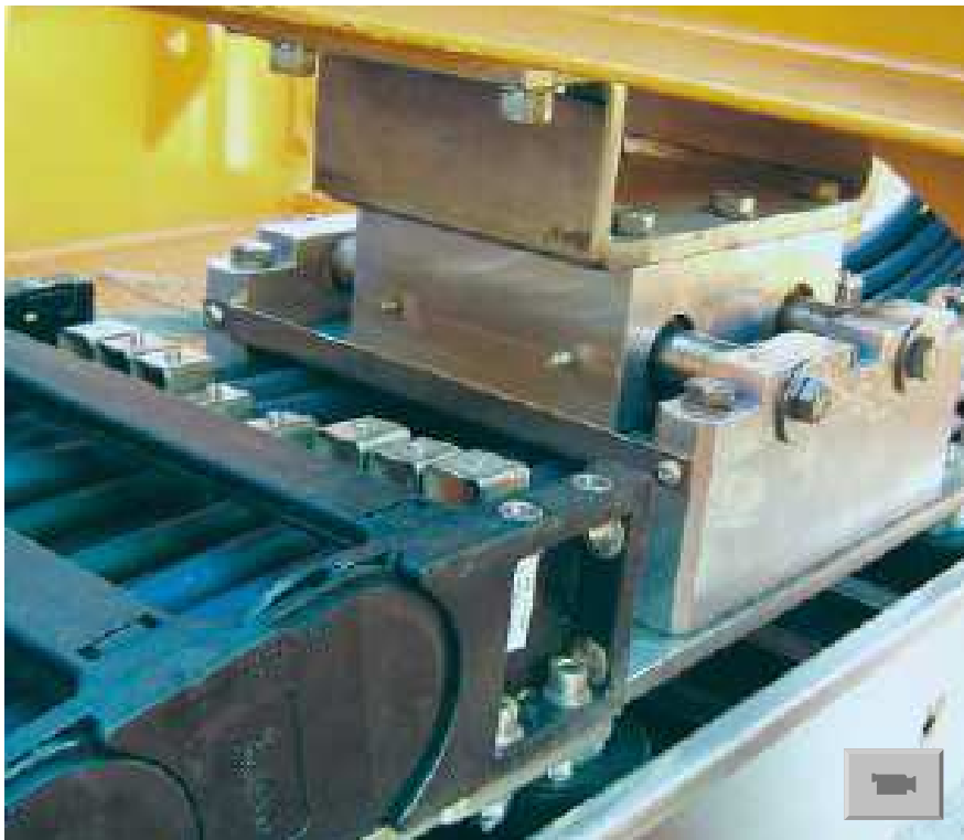
igus® floating moving arm for compensation of the lateral mismatch
