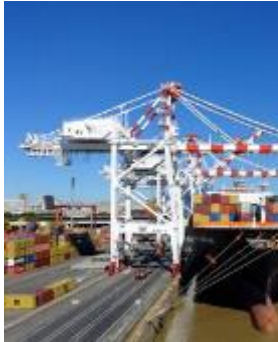
Buenos Aires, Argentina Boom extension and relocation of two non-Kalmar STS cranes ▪ 6-metre boom extension
